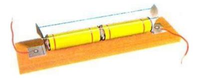
One of the reasons may be that the rubber band used in the cell holder may not be tight enough to keep the two cells in contact with each other. If the cells are not in proper contact with each
